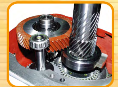
STRONG BACK GEAR TRANSMITTING INSTEAD OF TIMING BELT FOR HI-LO SPEED.(V-200)
