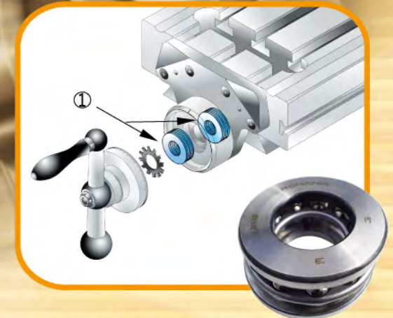
THRUST BEARINGS SUPPORT ON LEAD SCREWS 1. THRUST BEARINGS SUPPORT ON TABLE, SADDLE & KNEE TO PRE-LOAD THE FEED SCREWS (EXCEPT V-200)
