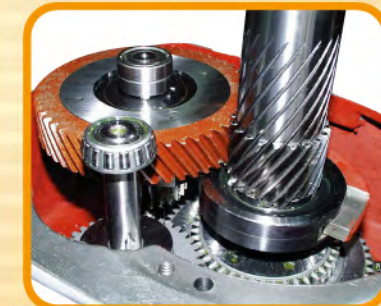
STRONG BACK GEAR TRANSMITTING INSTEAD OF TIMING BELT FOR HI-LO SPEED
