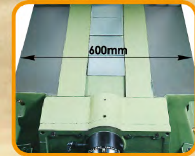
SUPER EXTRA SIZE BED WAY WIDTH 600MM(23.62") WITH HARDENED & GROUND.
