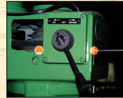
ADJUSTABLE BRAKE HANDLE INCREASES THE LIFE OF BREAK SHOE. (STEPHEAD)
