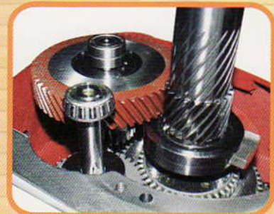
STRONG BACK GEAR TRANSMITTING INSTEAD OF TIMING BELT FOR HI-LO SPEED.(V-200)
