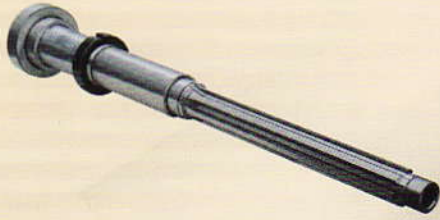
NST#40 SPINDLE MATERIAL SCM415 (SAE4115) FULL PIECE BY CARBONIZING & PRECISE GROUND.(V-200)
