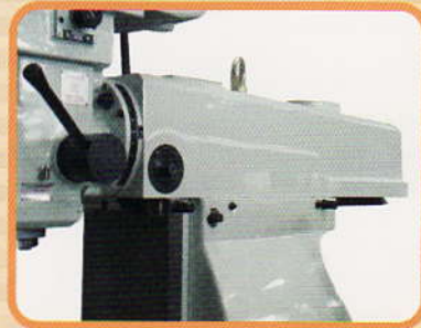
RAM DIRECT MOVE ON WIDE SLIDEWAY OF COLUMN.(V-200)
