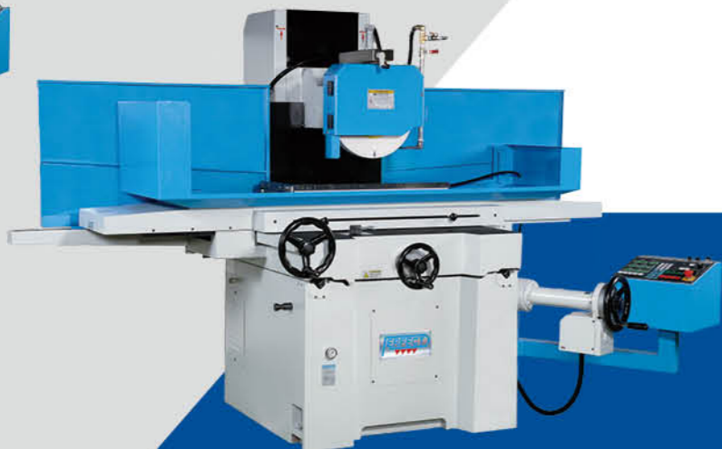
PFG-D4080AH 400x800mm Table surface +NC Auto down feed system, Parallel dresser, Back water splash shield (Option) • Hydraulic longitudinal feed Auto cross feed Manual vertical feed Table longitudinal travel is controlled by sensor and solenoid valve Continuous lubrication
