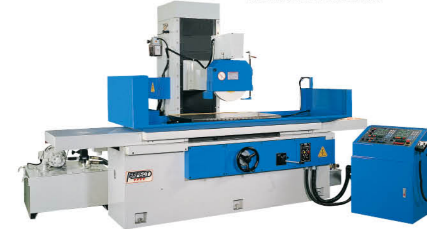
PFG-60100AHR 600x1000mm Table surface +NC Auto down feed system & NC Auto parallel dressing and compensating system (Option) • Hydraulic longitudinal feed Auto cross feed Vertical feed is driven by AC servo motor Table longitudinal travel is controlled by sensor and solenoid valve
