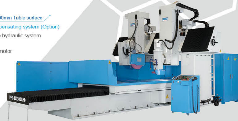
PFG-160300AHD 1600x3000mm Table surface +Vertical spindle head (Option) • Stepless variable proportional valve hydraulic system Cross & Vertical feed is driven by AC servo motor NC Auto down feed system
