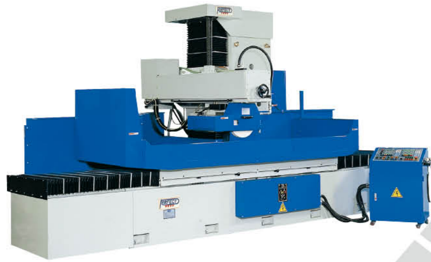
PFG-100200AHD 1000x2000mm Table surface +NC Auto parallel dressing and compensating system (Option) • Stepless variable proportional valve hydraulic system Auto cross feed Vertical feed is driven by AC servo motor NC Auto down feed system
